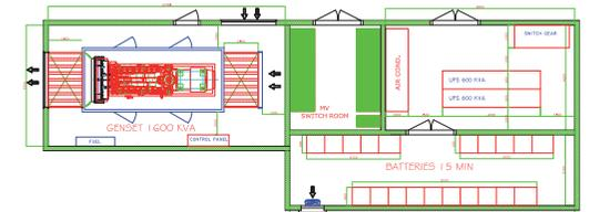
Static UPS system of 1200 kVA
